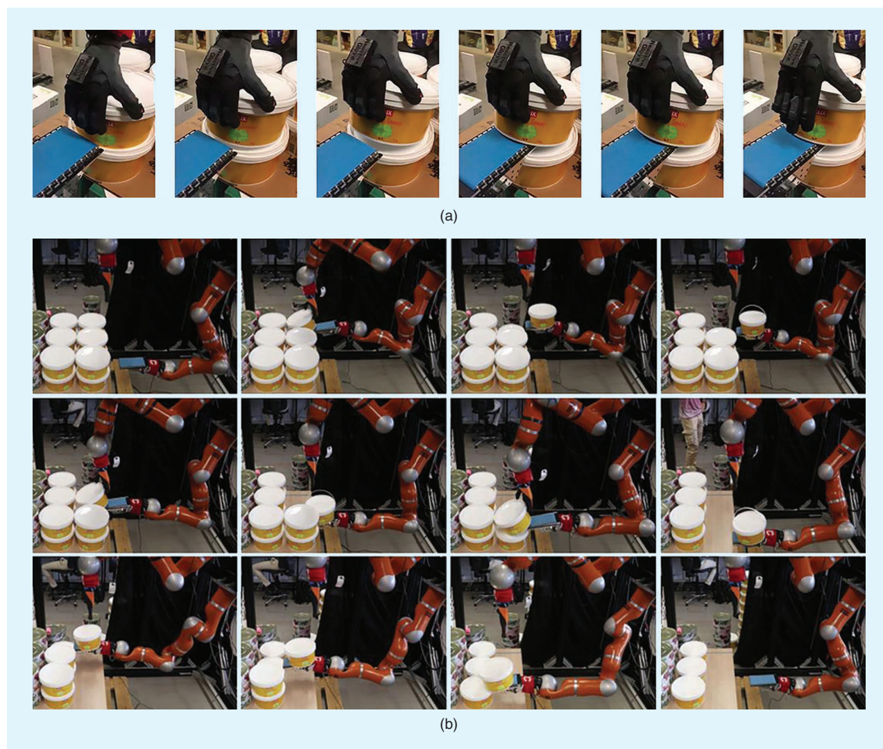
Figure 8. The WRAPP-up picking cylindrical objects. (a) The horizontal rotation primitive. (b) Cylindrical objects being picked using the horizontal rotation strategy.
