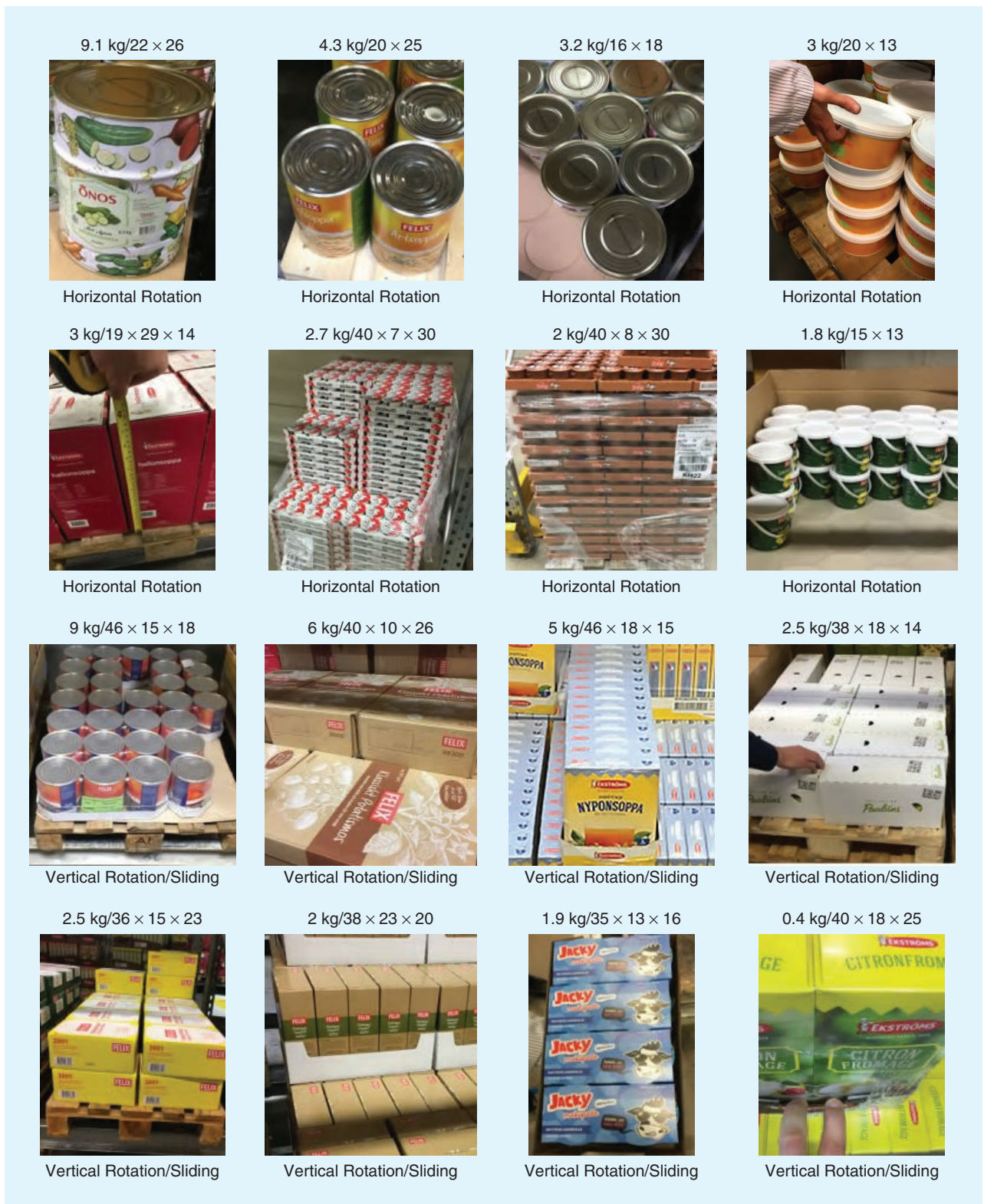
Figure 2. The objects considered for picking tasks, with their weight (in kg), size (in cm), and related grasping strategies.
